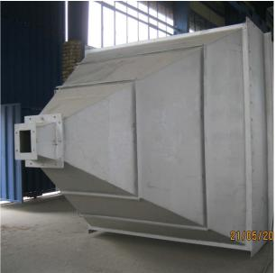
**Plenum:** The outlet plenum can be either open to roof top access or walk-in style. The top accesee configuration is ideal for indoor or tight budget applica-
